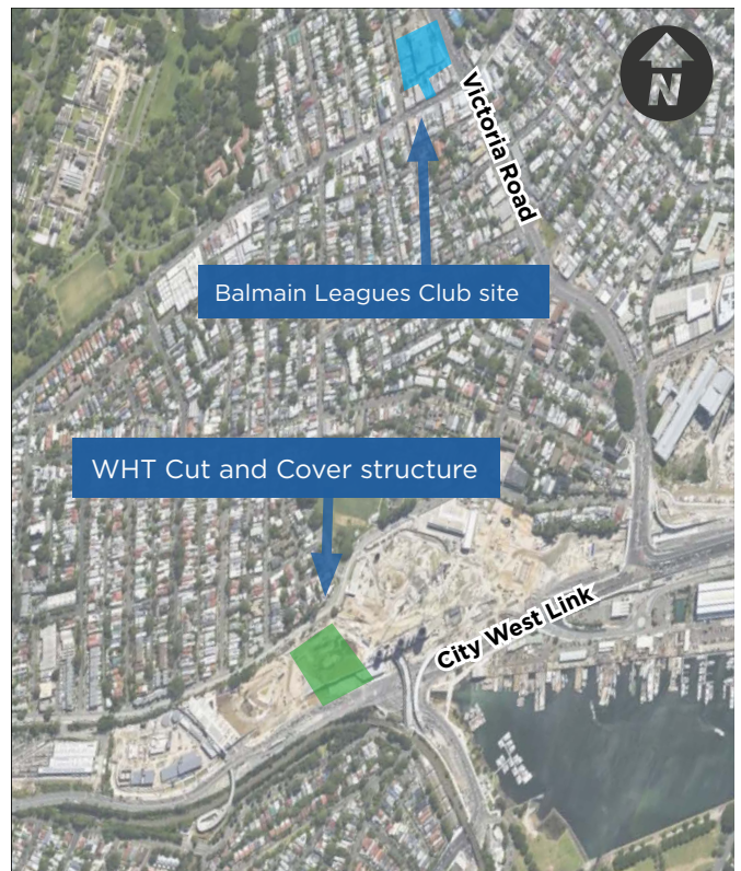
The new WHT support site (green) has fewer sensitive receivers than the original design (blue), and adjoins a major road (City West Link) that can better accommodate heavy vehicles.
